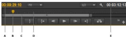
A. Current time display B. Playhead C. Zoom scroll bar D. Time Ruler E. Duration display
